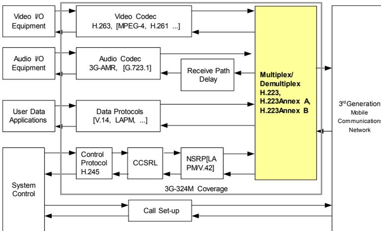
Fig. 1. Architecture of the 3G-324M protocol stack
