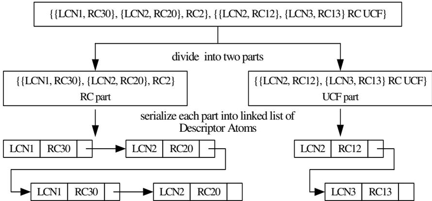
Fig. 3. Example of serialization
